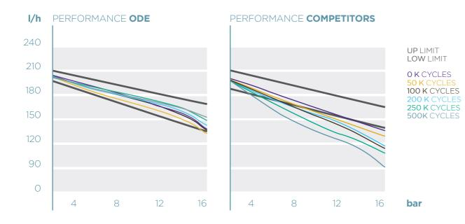
Opening the bypass without pressure drops with a more linear behavior.
